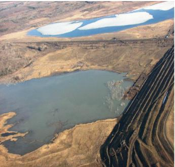
Bankrupt LTV Steel Mining Company tailings basin near Hoyt Lakes. PolyMet purchased both the crushing facilities and tailings basin for its proposed sulfide mine. PolyMet would layer more tailings on top of LTV tailings that are already leaching contaminants into the St. Louis River watershed.
